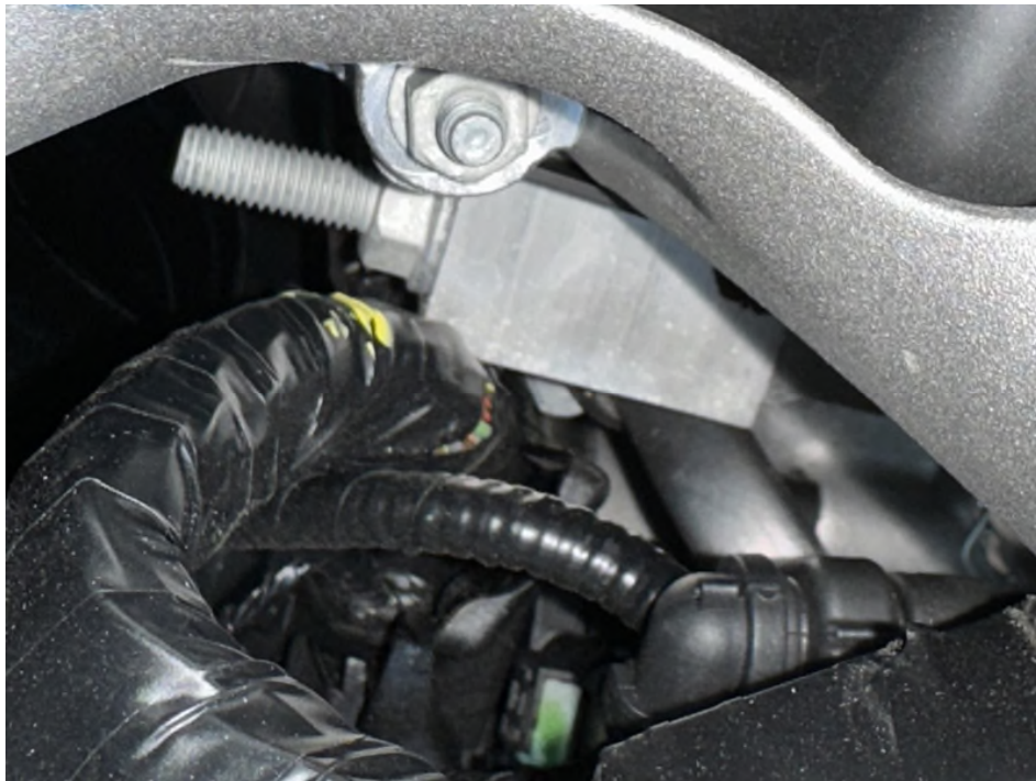
Fig. 8 AIS Y-Pipe near the lift stud
