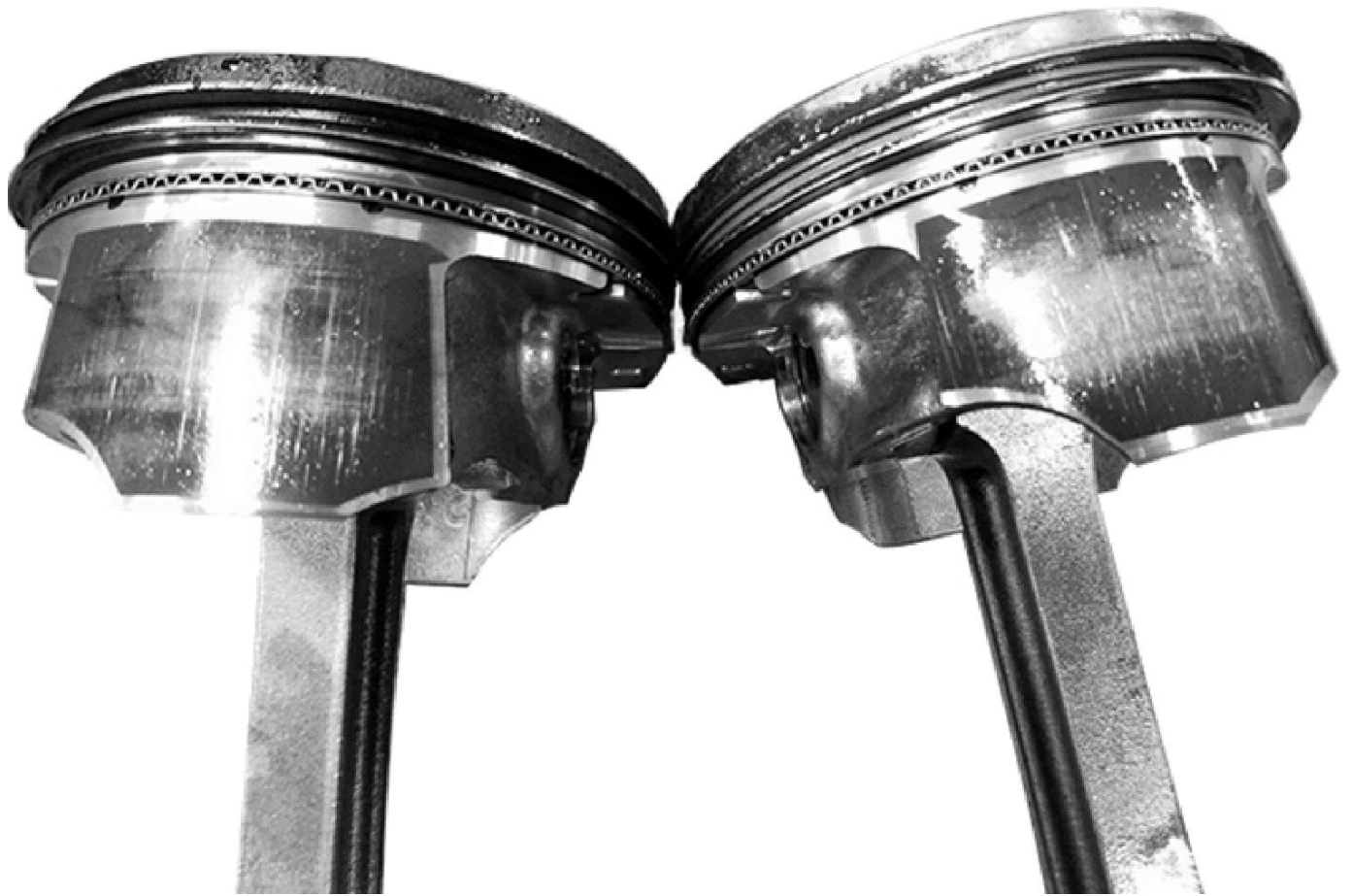
The piston skirt and piston ring damage caused by abrasive cleaning pads.
