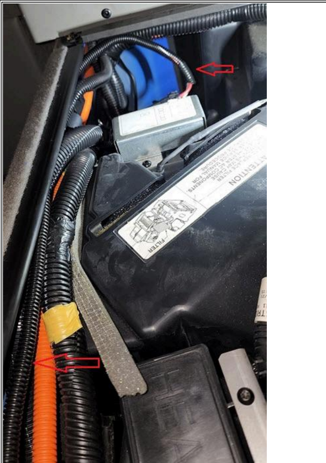
Figure 4: Routing of the 100B/C No-Idle System controller power sense/ground connector overlay
