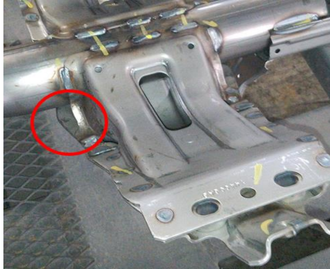
Fig 2. Area to inspect for wire chaffing. Note harness is not present.
