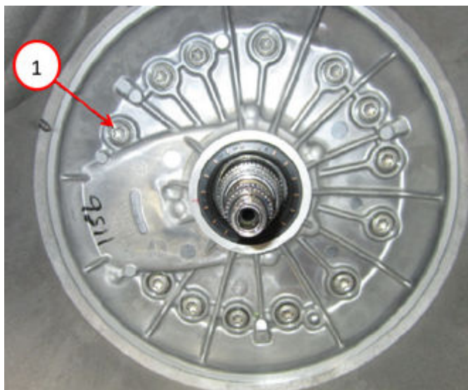
Fig. 14 Oil Pump Housing
