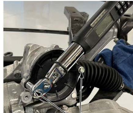
TORQUE BOLTS 8 N·m (6 lb-ft)
