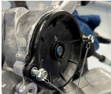
BOLTS Loosely install.
