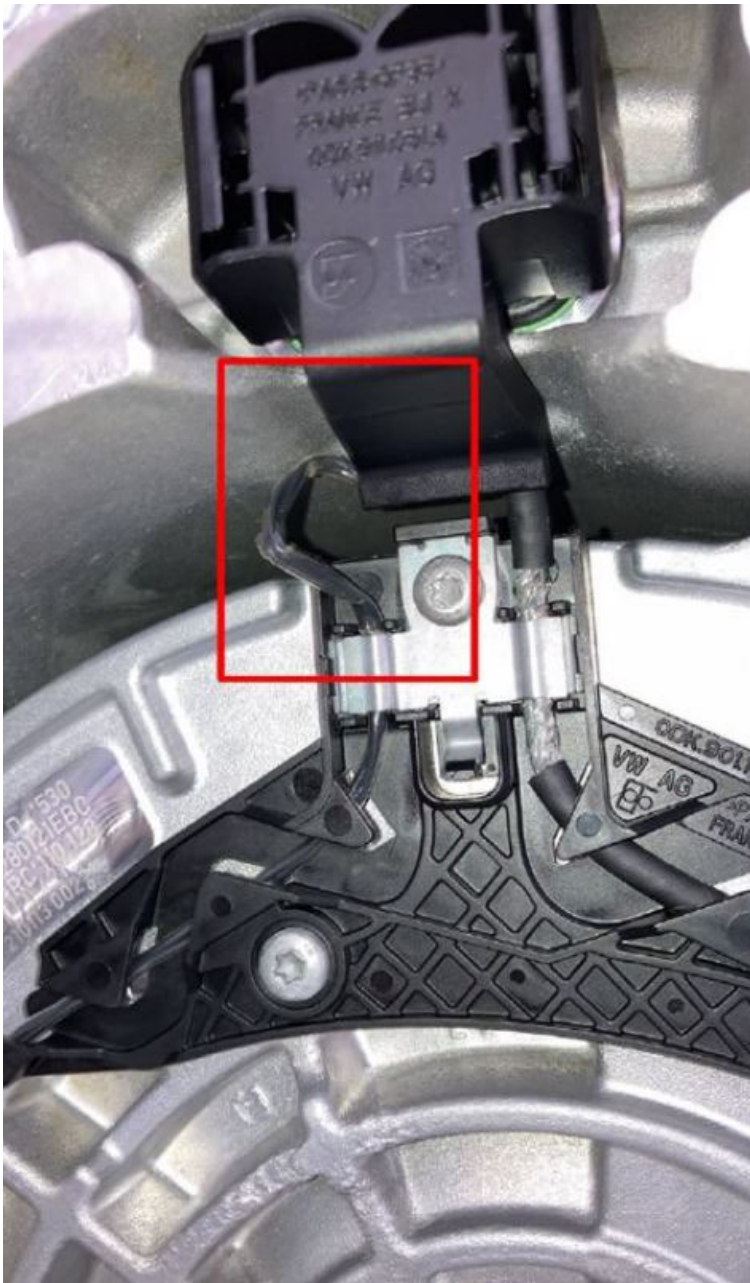
Figure 1. Wire not fitted correctly
