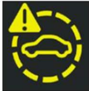
Figure 2: Symbol for “Audi pre sense not available at the moment” (MY2021 and onwards).
