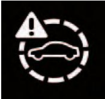
Figure 1: Symbol for “Audi pre sense not available at the moment”. (Up to MY2020)
