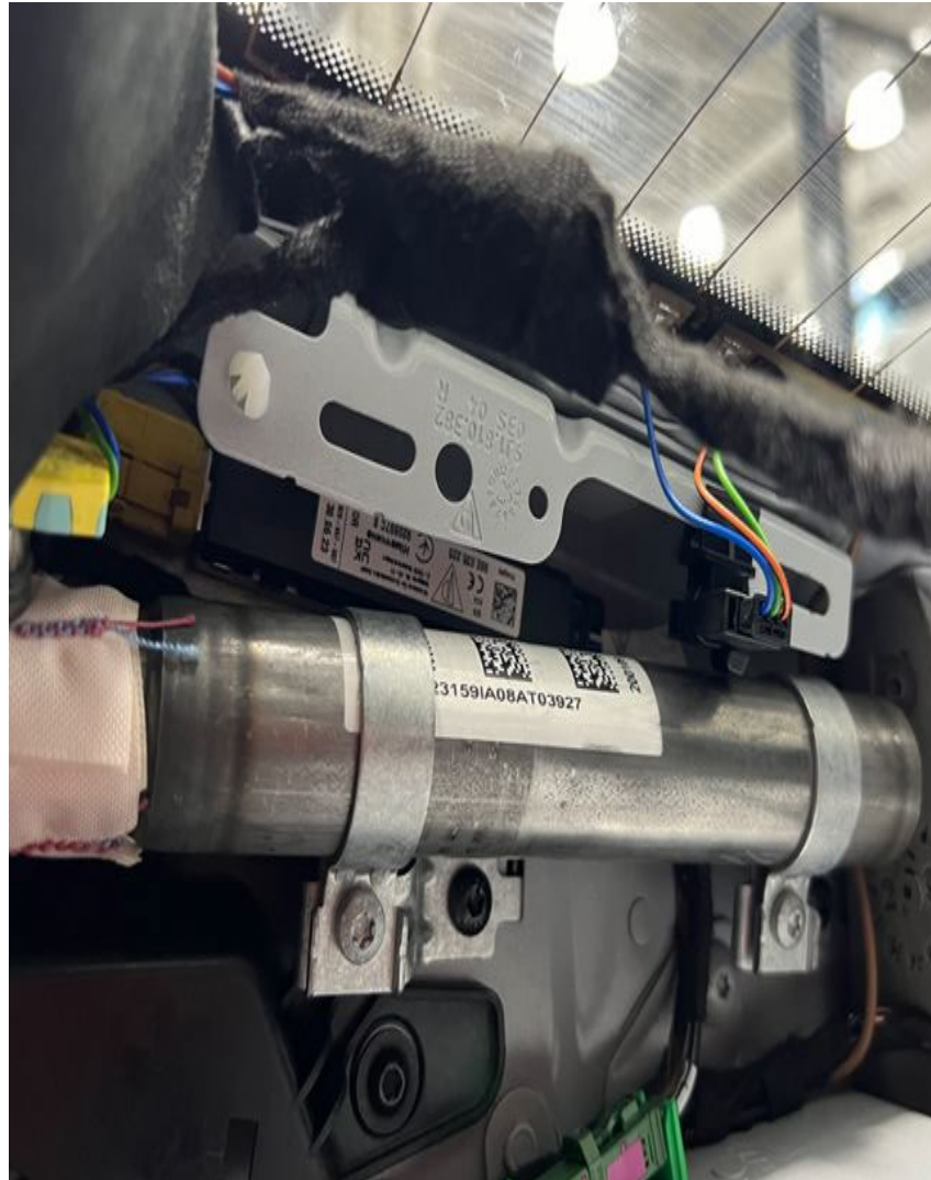
Figure 5: Insulate connector and harness.
