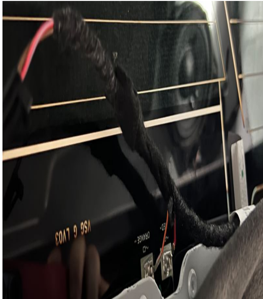
Figure 6: Insulate connector and harness.
