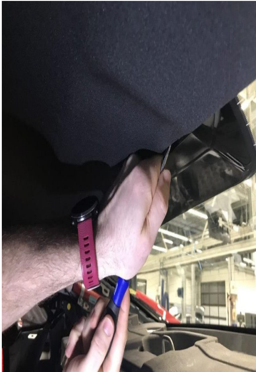
Figure 2: Remove 3 d brake light.
