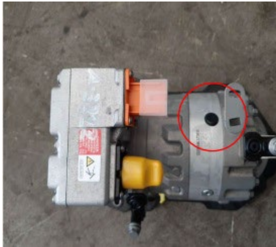
Figure 1. Pressure relief valve on the air conditioning compressor.
