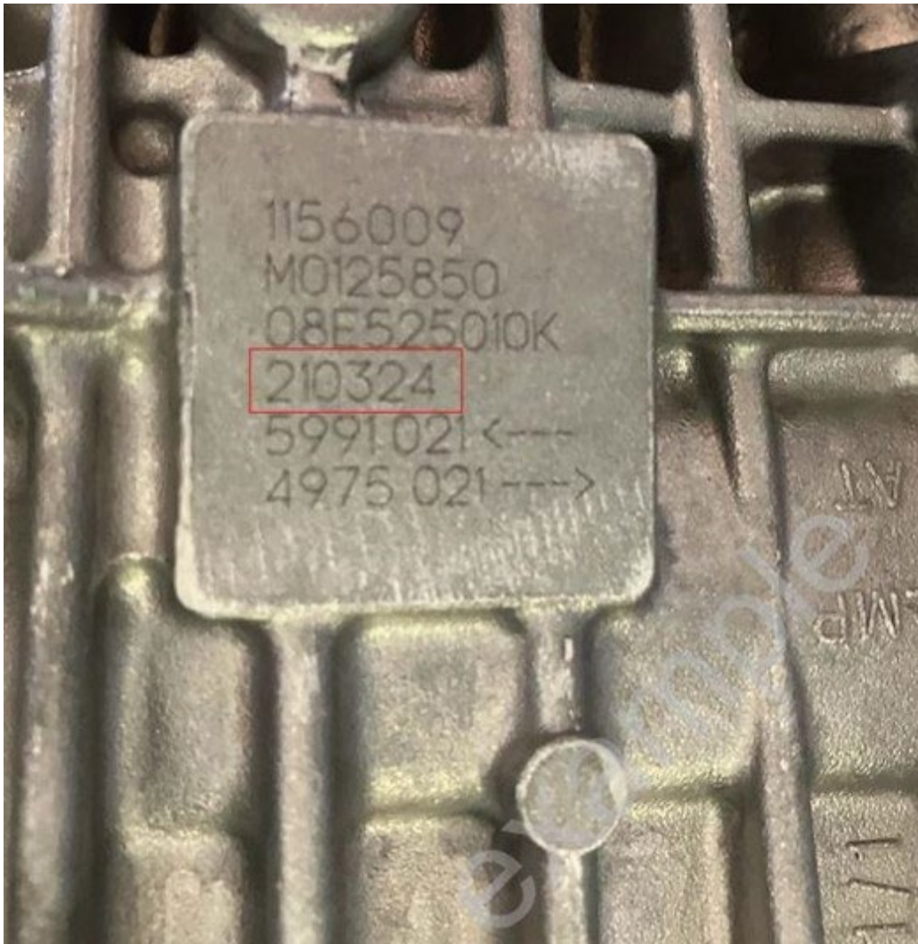
Figure 3. Example of engraving on underside of rear final drive: production date 03/21/2024.
