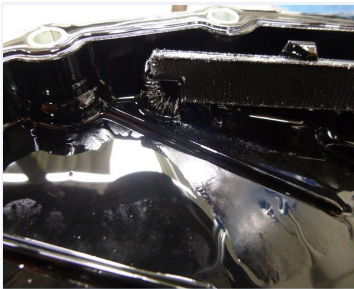
Figure 5. Abrasion is visible on the permanent magnets of the oil pan.
