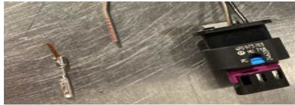
Figure 2: Wire damaged inside G31 connector
