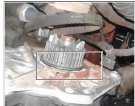
Leaks on the coolant pump close to the radial shaft seal ring
