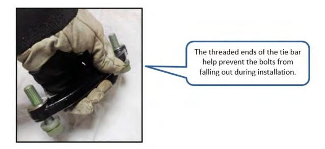
**STEP 12:** Reassemble the left front brake caliper bracket, caliper, and pads along with the tie bar and mounting bolts. Torque the mounting bolts to 142 Nm (104.7 ft-lb).
