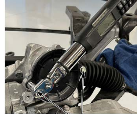
TORQUE BOLTS 8 N·m (6 lb-ft)
