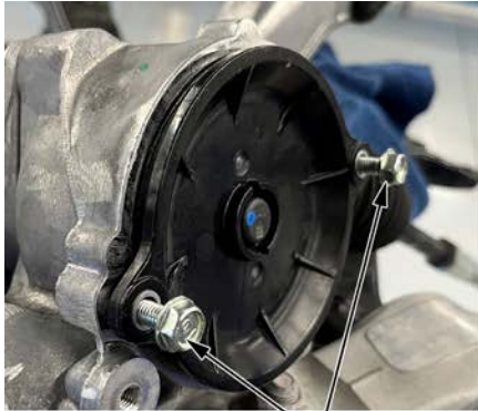
BOLTS Loosely install.
