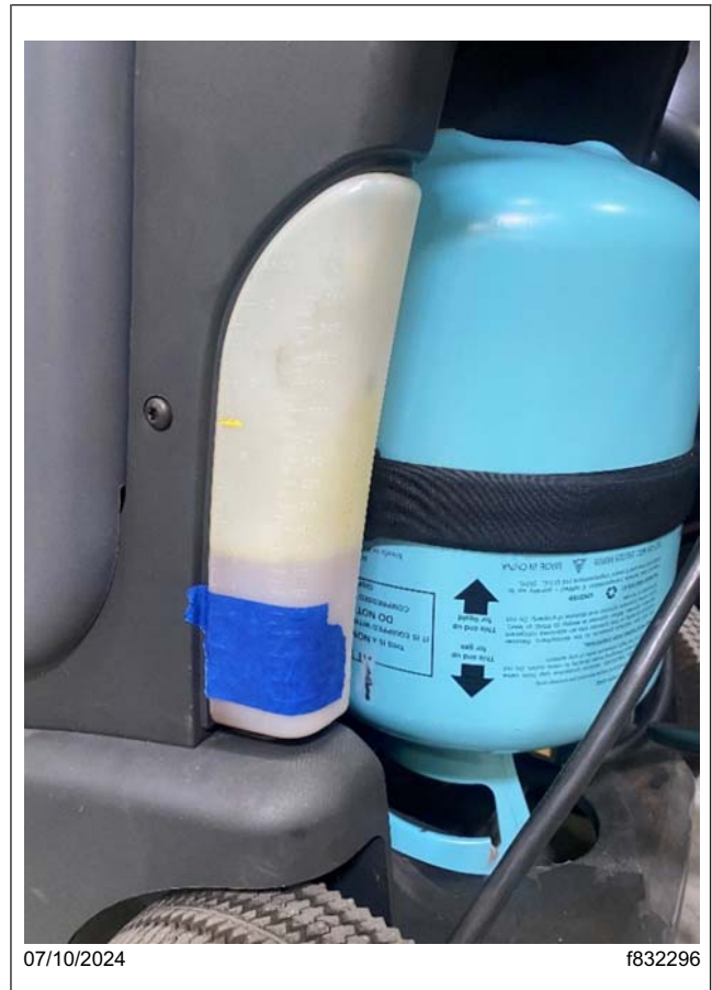
Fig. 3, Oil Recovered with the Refrigerant
