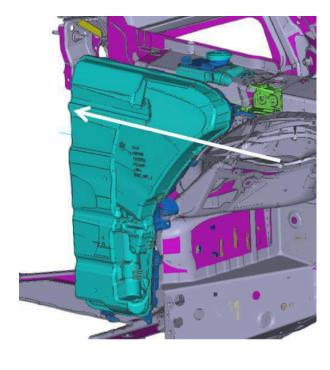
5. After guiding the washer fluid reservoir into the holder. Press the reservoir firmly towards the passenger compartment before tightening the self-locking hex bolt.
