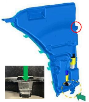
4. Before installing the new reservoir, apply two pieces of fabric tape to the upper mounting point (circled in red).
