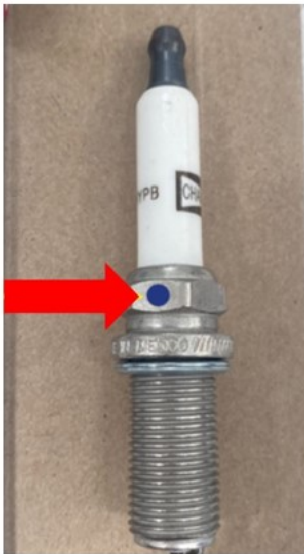
Fig. 1 Blue Mark On Re-Gapped Spark Plug
