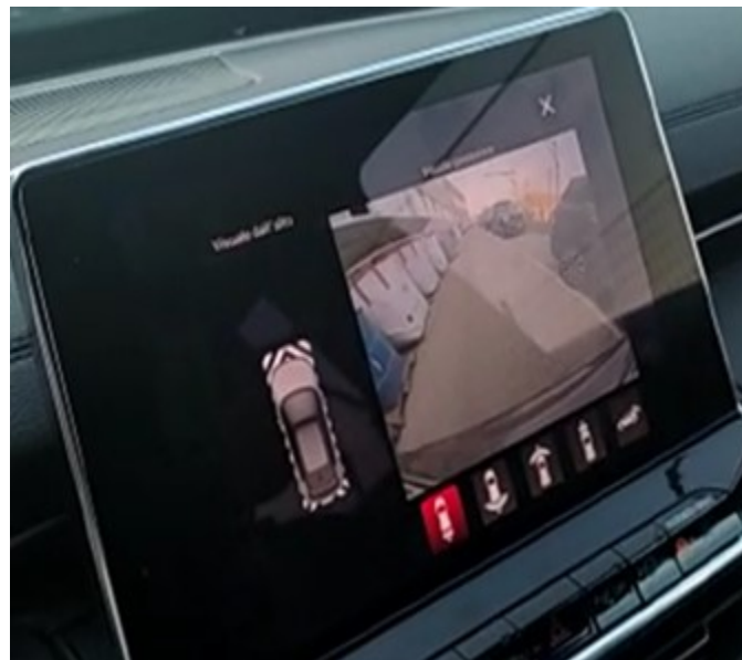
Fig. 1 Missing Gridlines When In Reverse Gear
