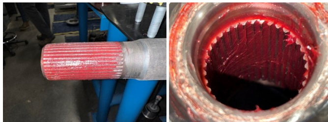
Fig. 3 Lubricated Axle Shaft/Hub splines
