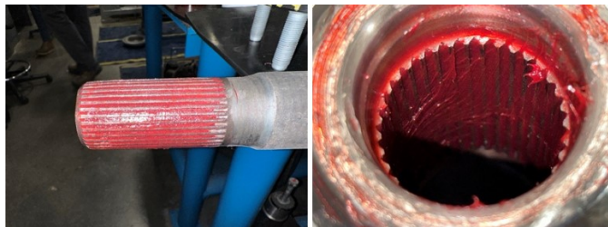
Fig. 3 Lubricated Axle Shaft/Hub splines
