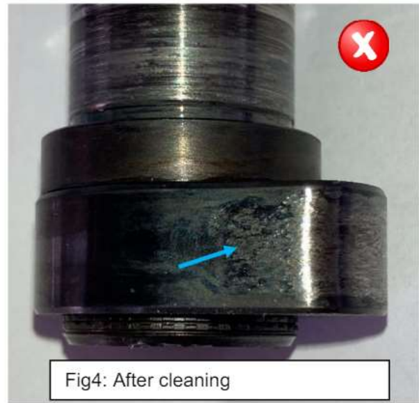
Fig. 3: Despite cleaning, a clearly perceptible run-in mark remains, camshaft is worn.
