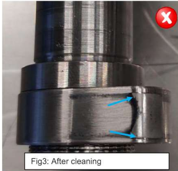
Fig. 3: Despite cleaning, a clearly perceptible run-in mark remains, camshaft is worn.
