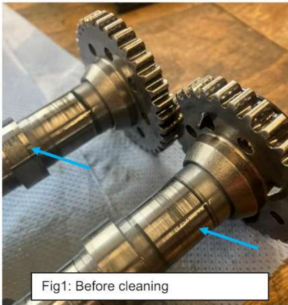
Fig. 1: Discoloration and marks immediately after removal from the engine.
