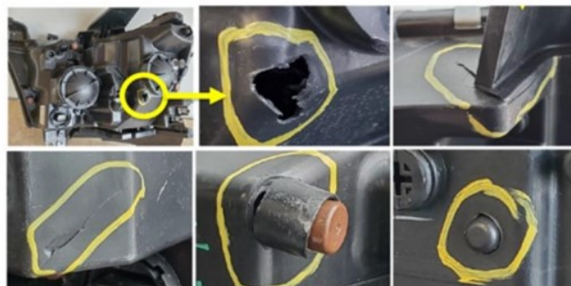
Fig. 3 Cracked, Damaged Or Broken Lamp Assembly Examples
