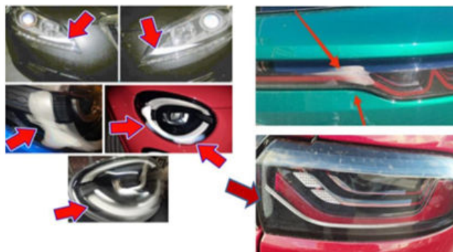
Fig. 1 Fogged Headlamp And Tail Lamp Assembly Examples
