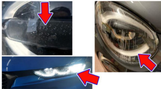
Fig. 2 Heavy Internal Moisture That Will Not Clear Examples
