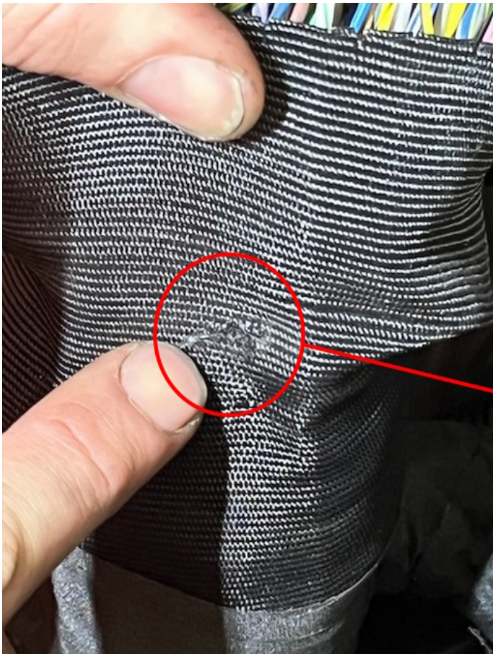
LM2 – Wiring Harness Contact at Alternator Bracket.
