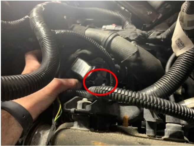
LM2 – TCCM Wiring Harness Contact at A/C Line and Bracket near Alternator.
