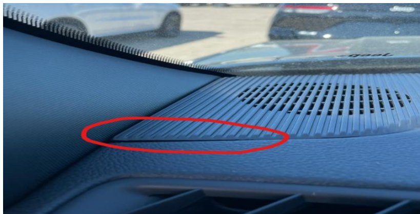
Fig 2 Gap In Corner(s) Of Grille.
