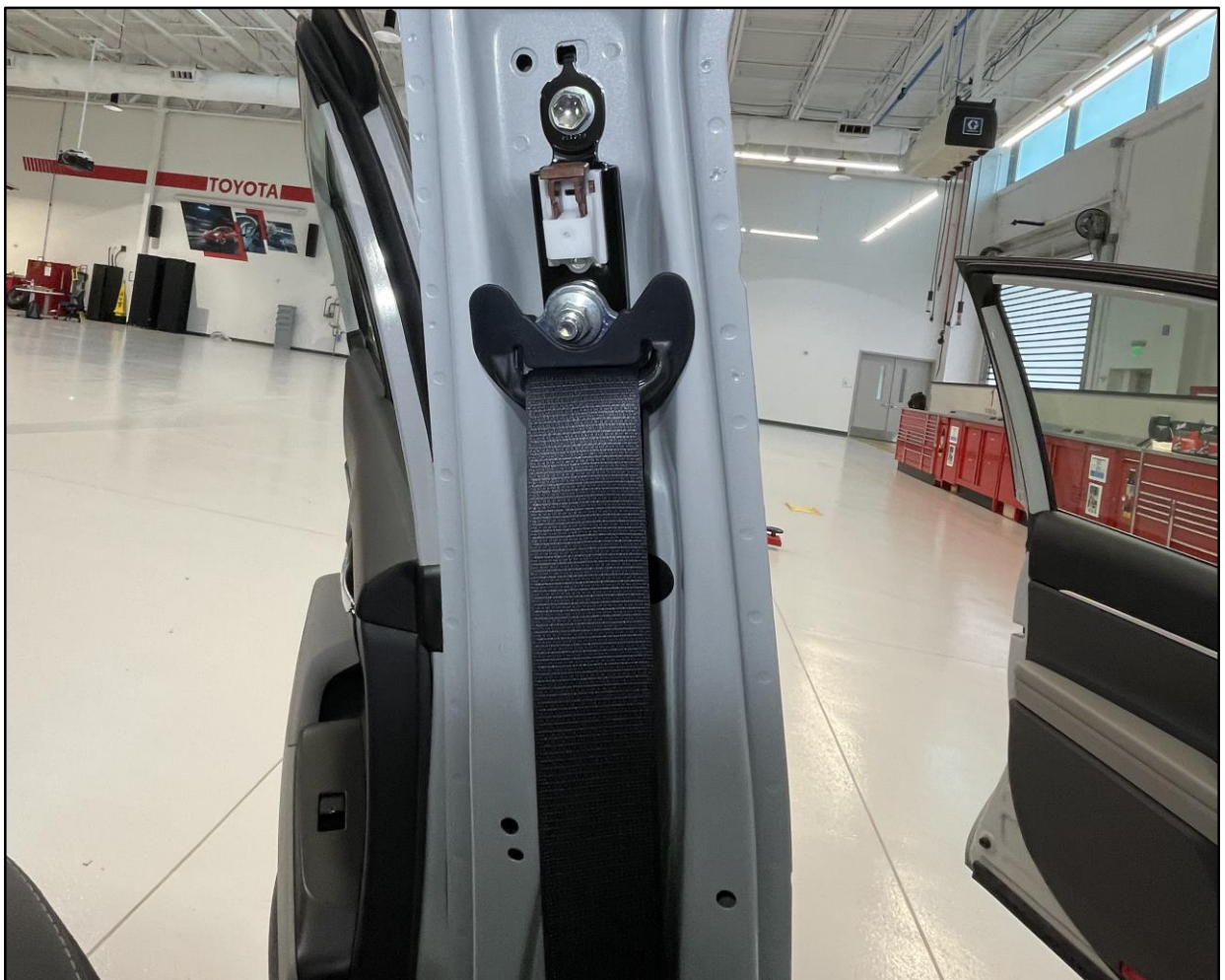
Figure 1. B-pillar After Removing Scuff Plate, Garnishes, and Weatherstrip
