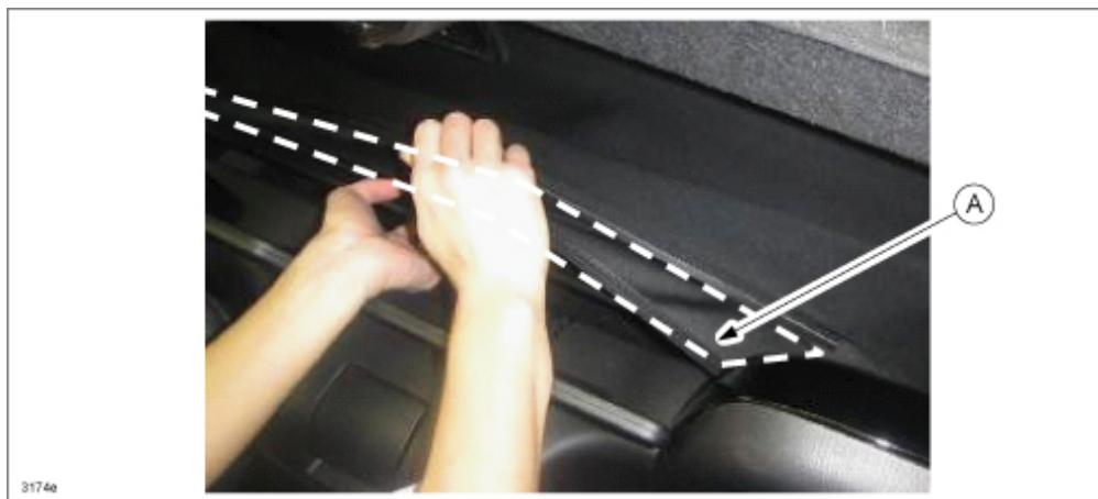
2) Turn over the resin edge of the tension cloth (A) to insert into the J-hook (B).
