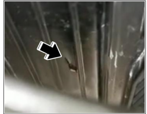
Crack in ATF pan
