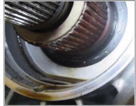
Oil leakage on output-shaft sealing ring
