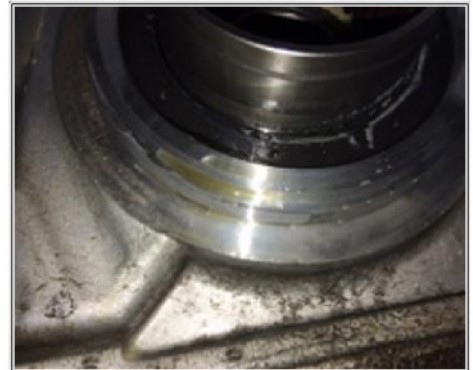
Oil leak on input-shaft radial shaft
