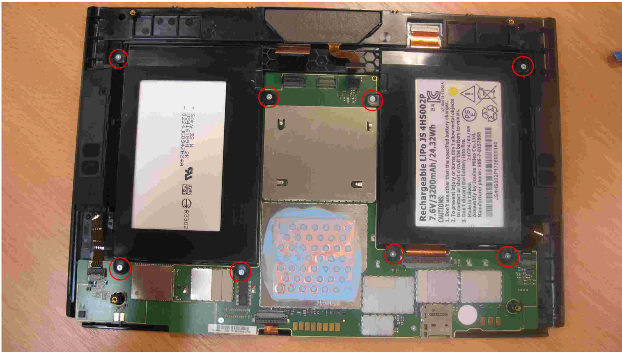
Figure 18. Remove the T3 Torx screws that secure the battery pack.
