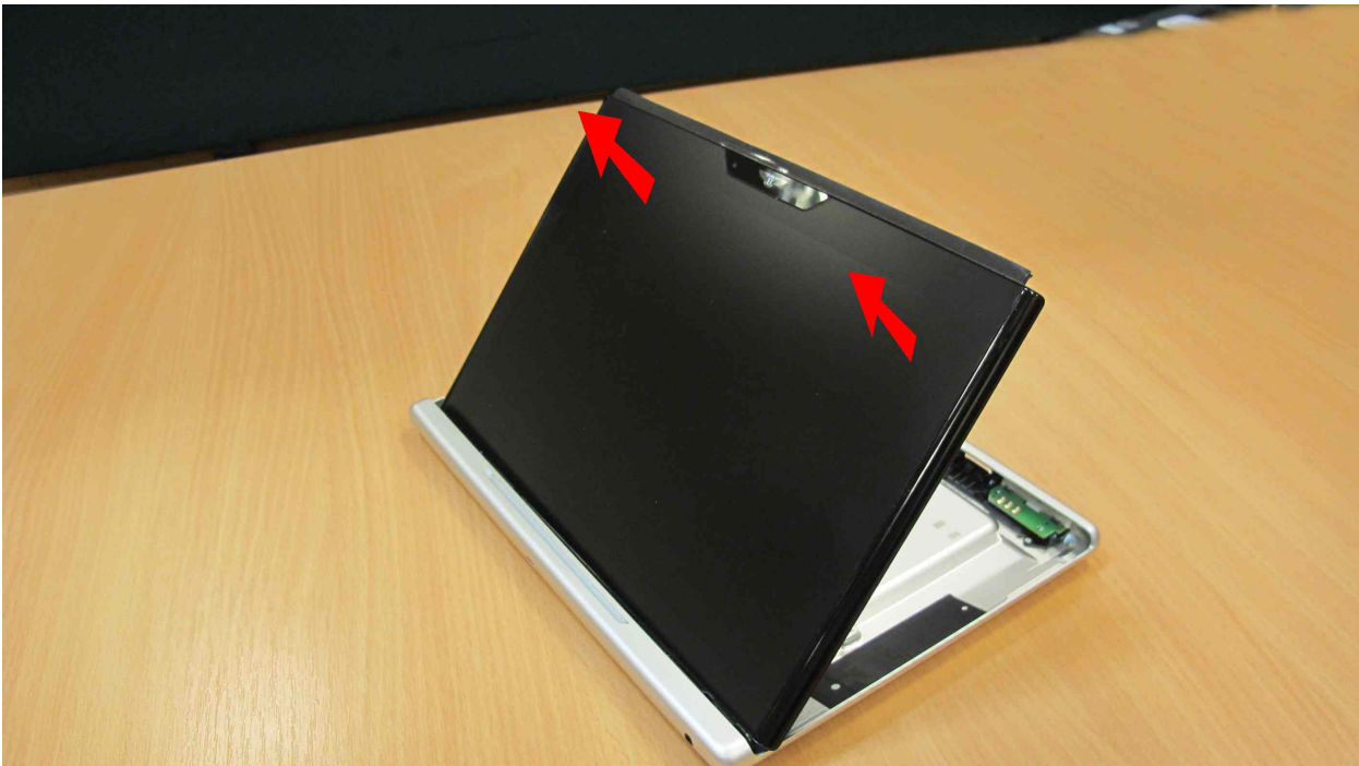
Figure 13. Lift the top edge of the screen to continue opening the tablet.
