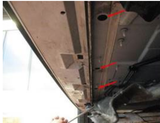
Figure 1. Access to the side member plugs.
