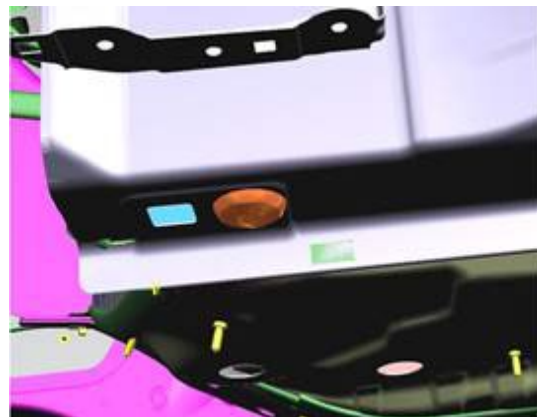
Figure 11. Drain plug on rear of the side member.
