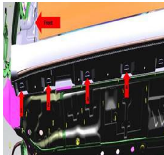
Figure 3. Sill trim fastener openings.
