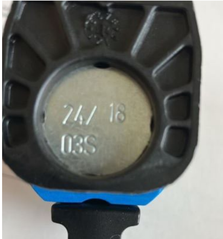
Figure 2. Door arrester of the improved type by date and version.
