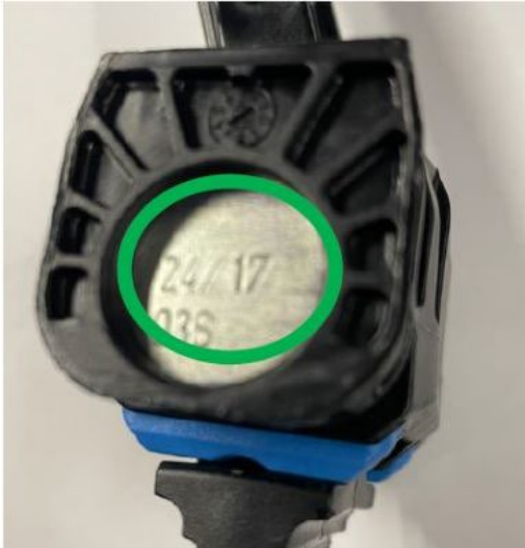
Figure 1. Location on the door arrester of the production date and part version.
