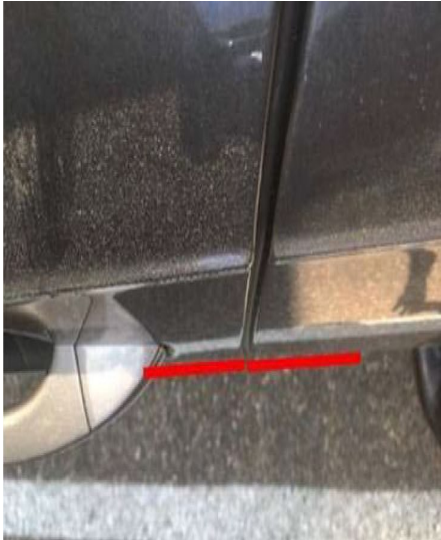
Figure 2. The front door can be flush or slightly under flush to the rear door.
