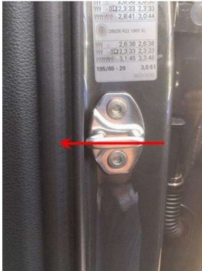
Figure 1. Adjust door striker inward by at least 0.5 mm.
