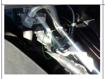
Mount a spacer (part number 11 53 7 537 923) in the engine compartment between the coolant hose feed and coolant hose return. The coolant hoses have to be turned about 10 to 15 degrees in the direction of the bulkhead.
