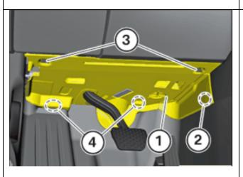
If the complaint still occurs after installing the spacer, the following must also be done: Remove the trim panel for pedal mechanism. See repair instructions REP 5145186
