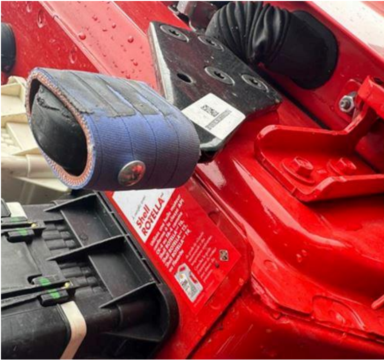
Figure #5: Rubber hose section over rubber hood stop shown as an alternate repair option.
