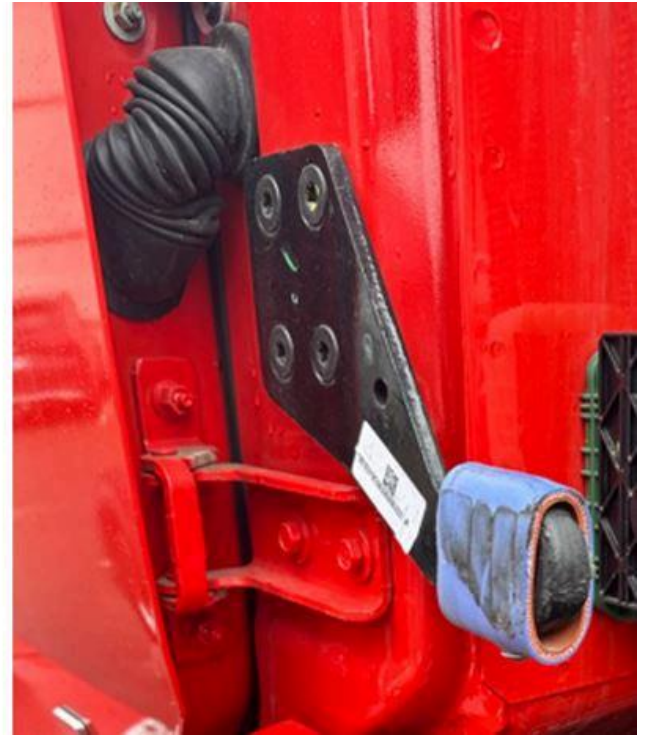
Figure #5: Rubber hose section over rubber hood stop shown as an alternate repair option.
