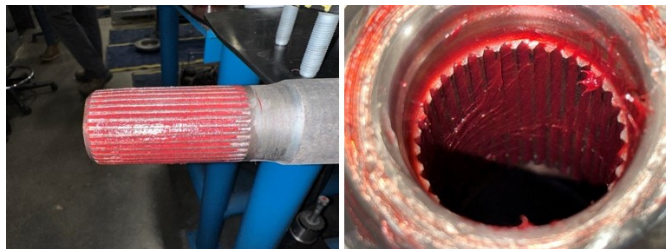
Fig. 3 Lubricated Axle Shaft / Hub splines
