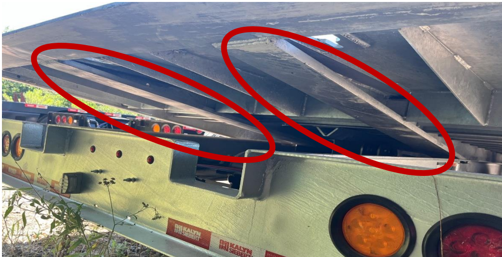
Main Beams underneath transition plate
