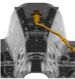
Replace the condensation water drain.
