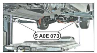
Remove High Voltage Battery unit as per Repair Instruction **61 25 010**
