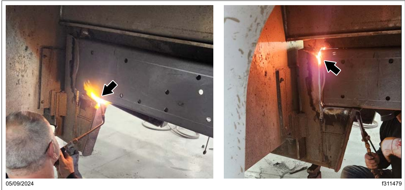
Fig. 37, Preheating to 150-Degree Fahrenheit
