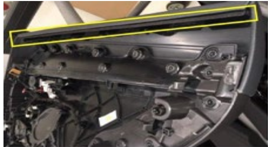
Figure 4. Fleece tape applied to mounting strip.
