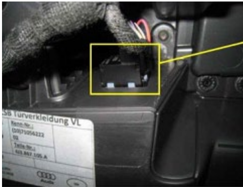
Figure 21. Apply fleece tape to pocket lighting.
