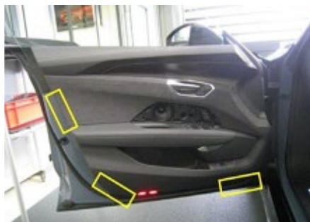
Figure 14: Apply felt tape to edge of trim panel.
