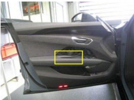
Figure 8. Isolate pull handle from armrest.
