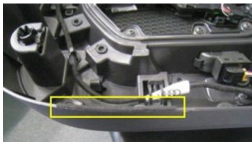
Figure 15. Felt tape installed on trim panel.
