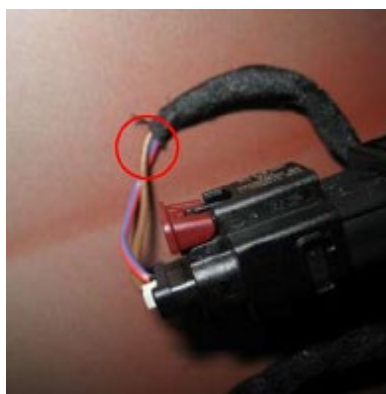
Figure 13. Wire harness contacting body.
