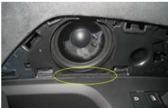
Figure 1. Felt strip section applied to opening in door panel.
