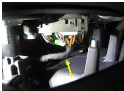
Figure 11. Wire harness contacting door trim panel.
