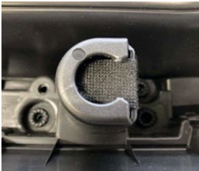
Figure 6. Door clip with fleece tape applied.
