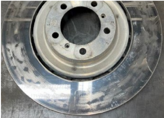
Figure 1. Brake disc with hotspots
