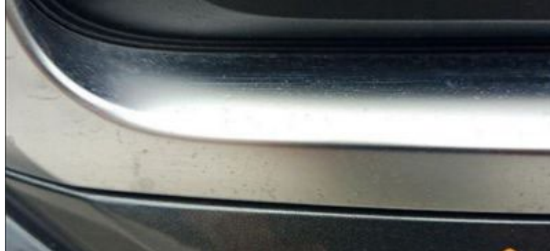
Figure 5. Spotting discoloration on the side cooling air grille trim.
