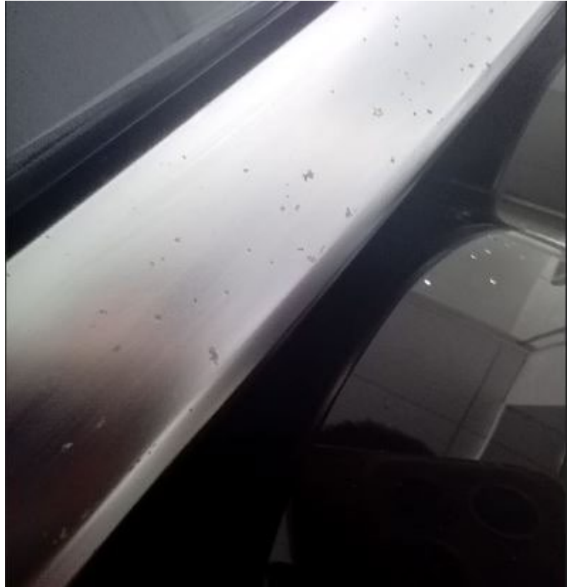
Figure 2. Pitting in the radiator grille trim.
