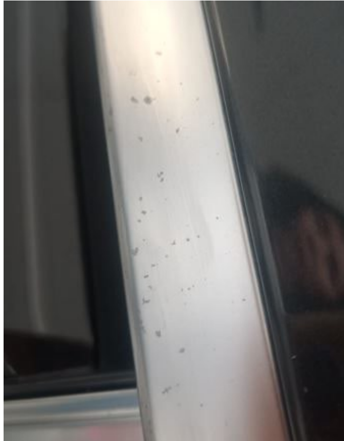
Figure 3. Pitting / spotting in the radiator grille trim.
