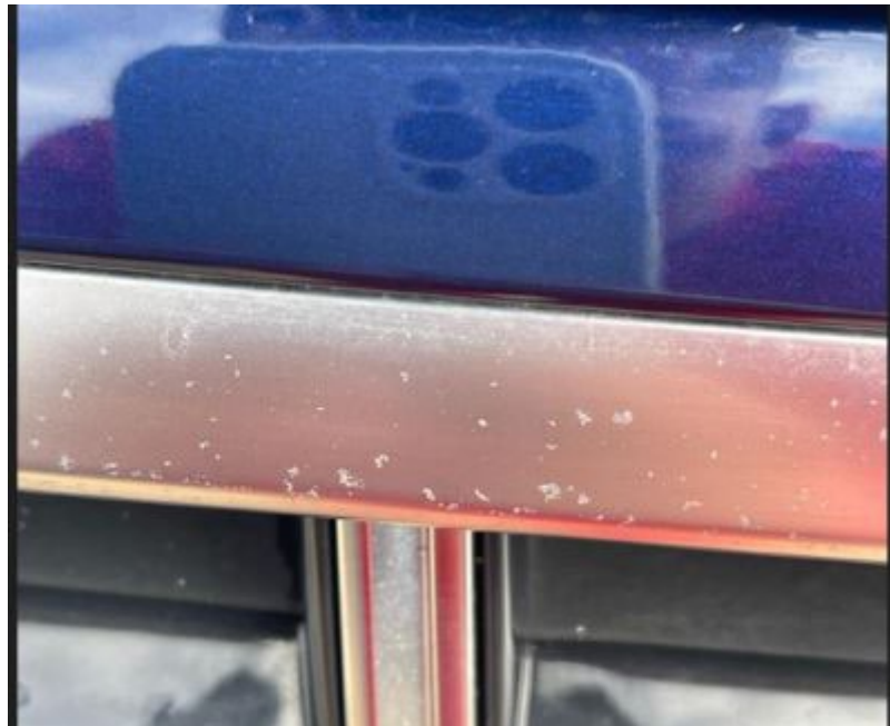
Figure 3. Pitting / spotting in the radiator grille trim.
