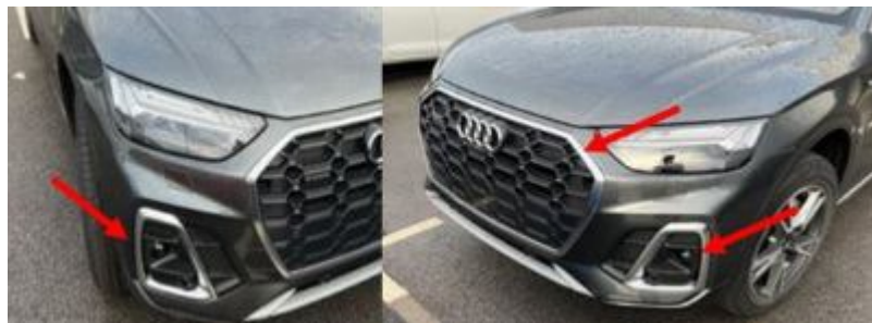
Figure 1. Areas of the front fascia showing damage.
