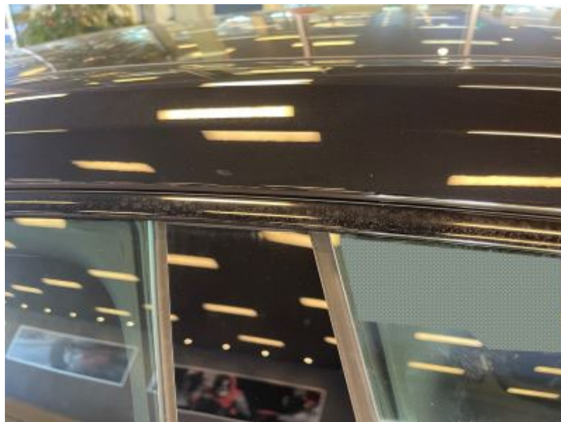
Figure 1. Typical spotting on black optic trim.
