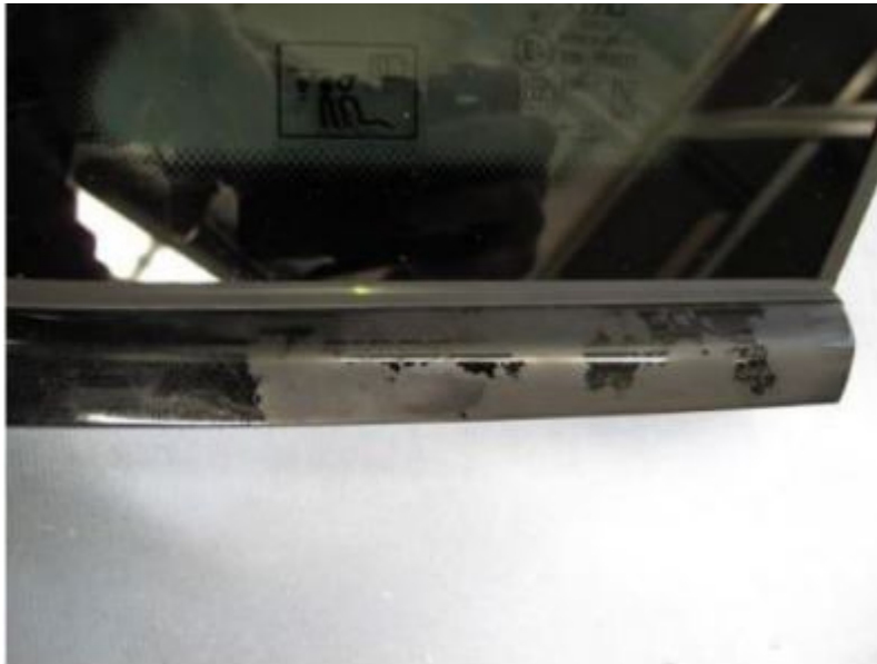
Figure 3. Black optic door trim peeling.
