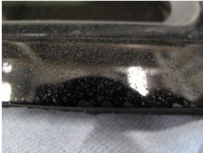
Figure 4. Droplet patterned finish adhesion failure.
