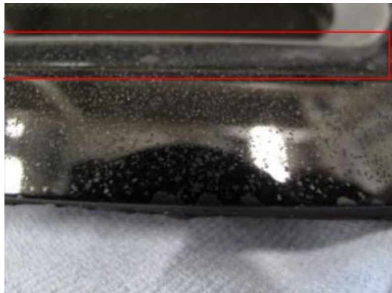
Figure 5. Droplet pattern migration to adjacent rubber strip.
