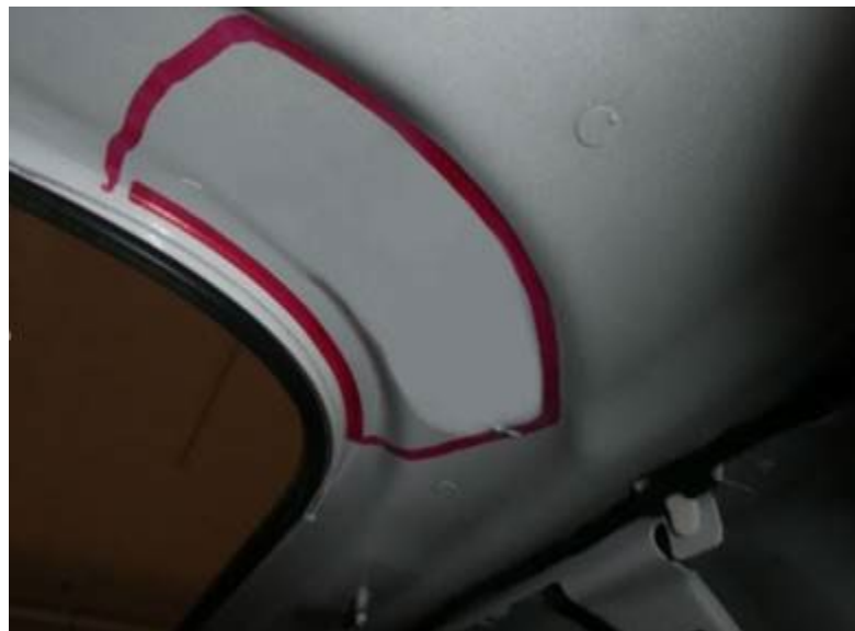
Figure 1. Right rear area of the sunroof opening to be reworked.
