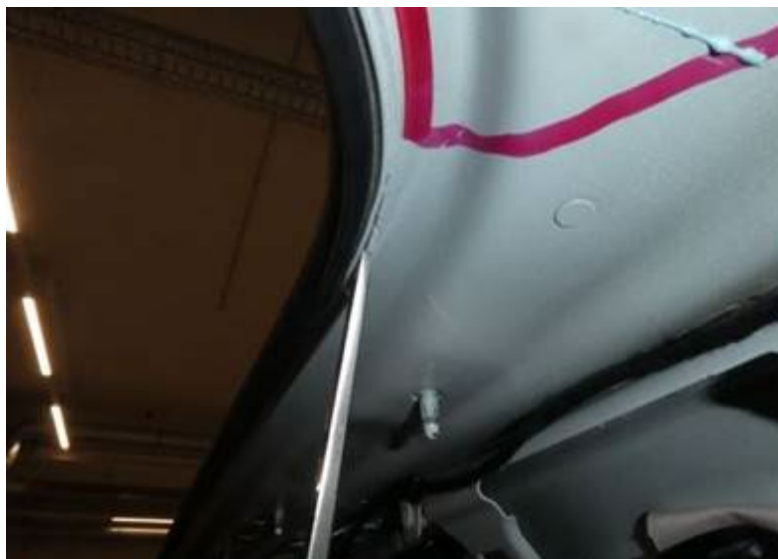
Figure 7. Adhesive joint separated.
