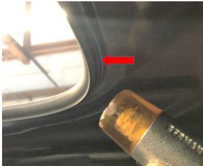
Figure 6. Area of sheet metal to strike with a plastic mallet.
