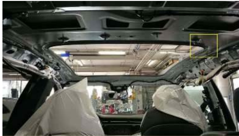
Figure 1. Right rear area of the sunroof opening to be reworked.
