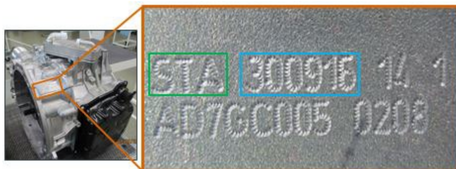
Figure 2. Transmission identification example.
