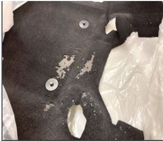
Fig. 2 Front Right Floor Carpet Deterioration
