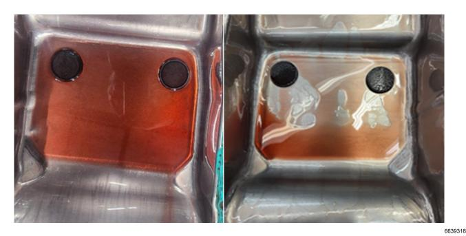
The fluid in the graphic above shows good color with no evidence of clutch material. This unit should be serviced with a valve body.
