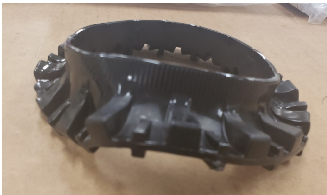
Fig. 2 Distorted Upper Isolator Spring
