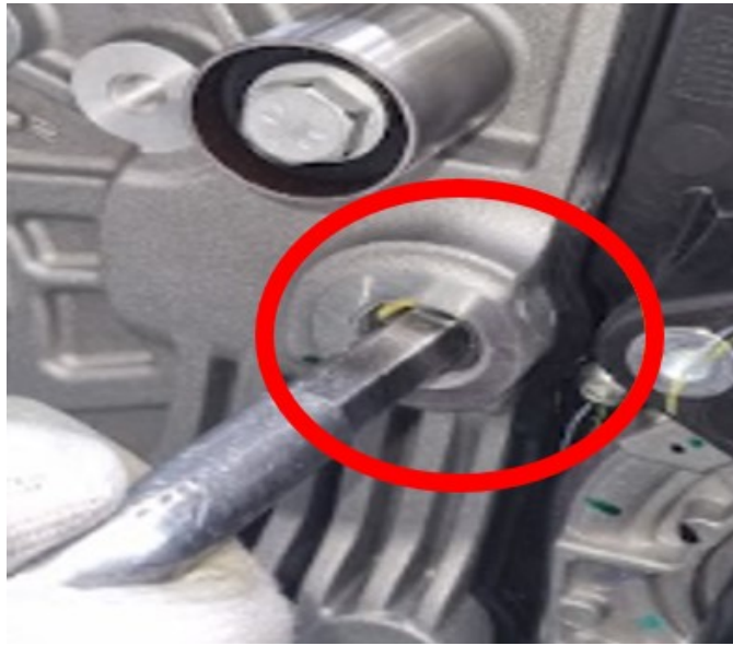
Fig. 3 Puma Bolt Loosening
